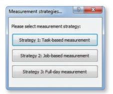
The Supervisor software provides complete tool for determination of occupational noise exposure from noise level measurements. The Supervisor provides automatic calculation of all required measurement results and uncertainties in accordance to three measurement strategies described in ISO 9612: task-based, job-based and full-day.
