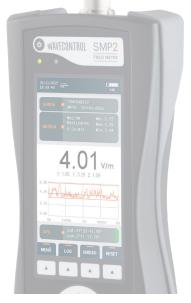
(\*) The frequency response can be corrected with the SMP2 by using the correction factors stored in the probe (ISO 17025 accredited calibration).
