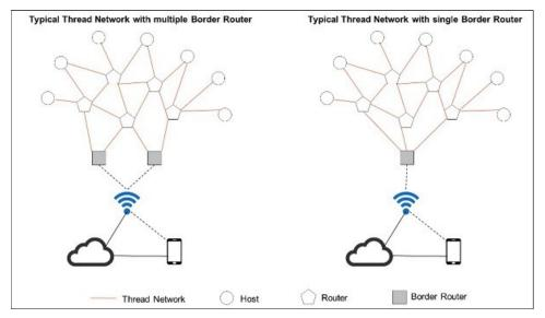
The Thread protocol allows the connection and communication of the Sphensor<sup>™</sup> data logger sensor network to one or more Sphensor Gateways.
