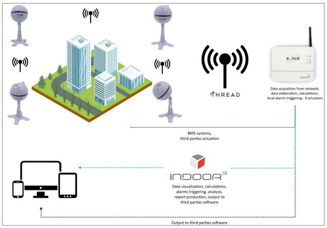
The **Sphensor**<sup>TM</sup> data logger sensors form an indoor sensor network and communicate with each other and with the Sphensor Gateway via **2.4 GHz radio**, **Thread protocol**. The Sphensor Gateway (TXRGB1101) with **dual antenna** can receive signals from sensors that communicate on the **868 MHz frequency** (see Table "Additional sensors integration").
